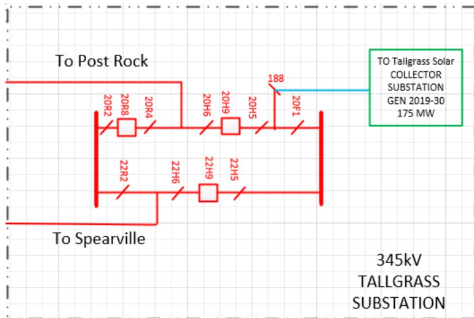
**Figure 1 GEN-2022-075 ITCGP Interconnection Substation One Line**
